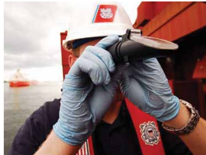
Figure 1b. A Ballast Water Working Group inspector using a refractometer to measure the salinity of the water from a ballast water tank.
