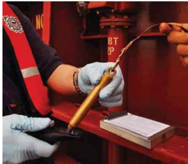
Figure 1a. Ballast Water Working Group inspectors placing water from a ballast water tank onto a refractometer during an Enhanced Seaway Inspection. A refractometer is used to determine the salinity of a liquid by measuring its refractive index.
