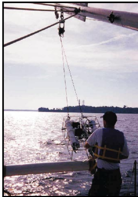
Figure 1. Seabird CTD datalogger being deployed from the stern of the RV Aquarius of the Great Lakes Center at Buffalo State College
