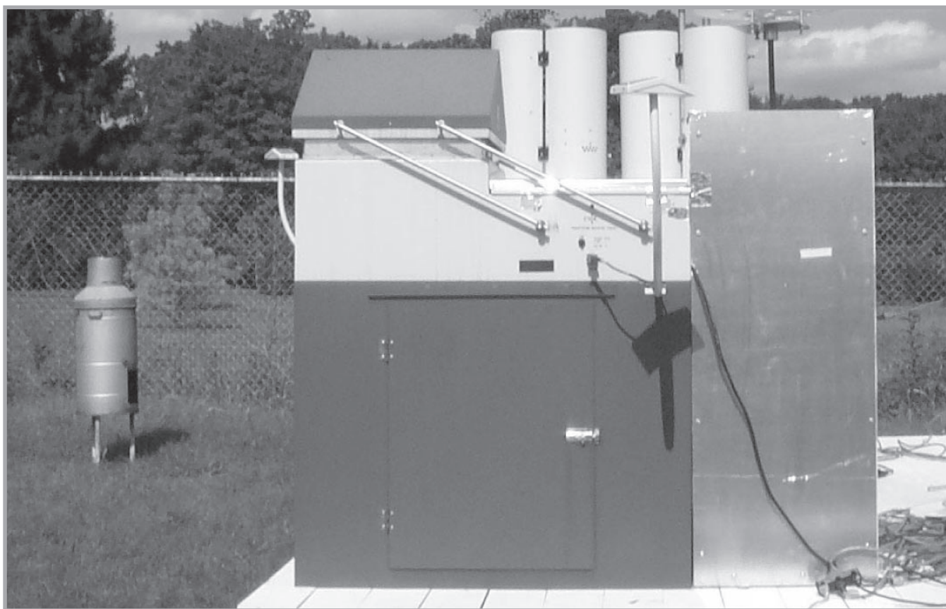
Figure 1. Modified MIC-B precipitation collector containing the dry deposition module and surrogate surface.
