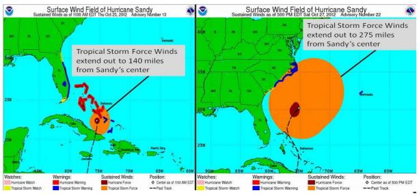
Figure 5: A comparison of the radius of tropical storm force winds between NHC Advisory #13 and #22 (operational data vs. post-storm analysis). *Source: NHC*
