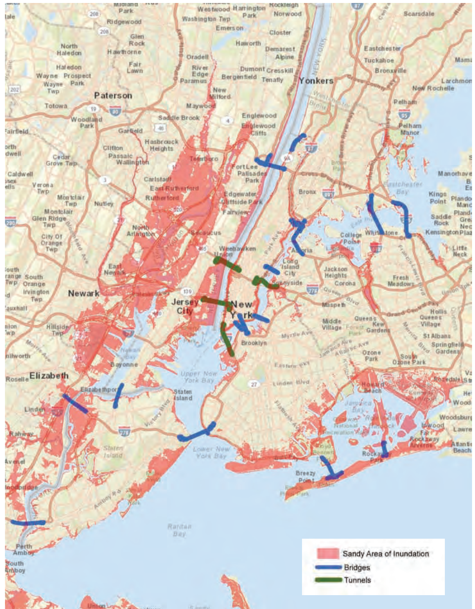
Figure T-14: New York City tunnels and bridges at risk of flooding. (FEMA, MTA, NJ DEP GIS, NYSDOT, NYCDOT, PANYNJ, 2012)
