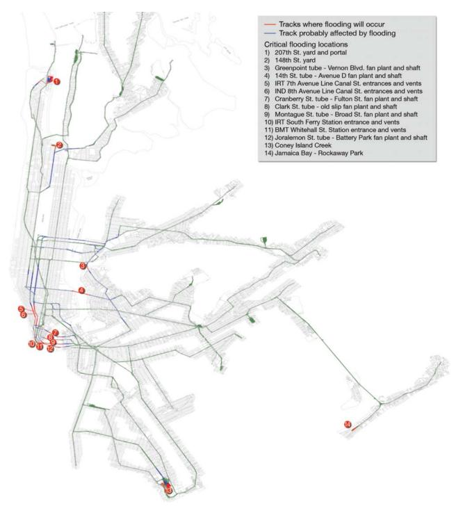
Note: Red symbols indicate definite flooding, blue ones potential flooding, the latter corresponding closely to the "overflow" segments in Figures 9.11–13. Green areas near the line tracks indicate locations of yards. Two yards along the Harlem River (upper left) are flooded, and so are facilities in Coney Island and Rockaway (bottom center and right). Source: MTA—NYCT, 2006, A. Cabrera (see Endnote 35)
