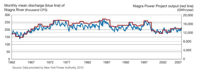
Figure 8.10 Comparison of power output levels of Niagara Power Project and monthly mean discharge rate of Niagara River (1962–2006)
