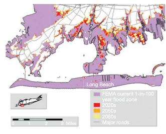
Figure 5.18 1-in-100-year flood zone for Long Beach based on the GCM-based central range sea level rise scenario
