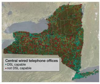
Distribution in 2010 of central offices for wired telephone in New York State. Those in green are capable of providing digital subscriber lines (DSL, 2009). Source: http://www.dslreports.com/comap/st/NY; basemap NASA
