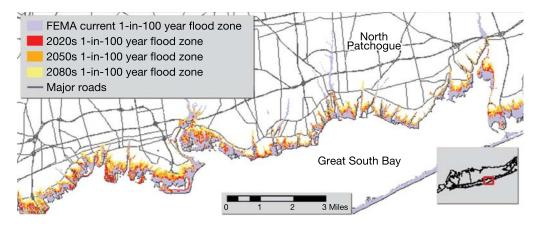
Figure 5.17 1-in-100-year flood zone for Great South Bay based on the rapid ice melt sea level rise scenario
