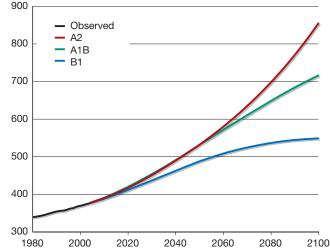
Based on IPCC emissions scenarios. Observed carbon dioxide concentrations through 2003 and future carbon dioxide concentrations in the A1B, A2, and B1 scenarios (2004 to 2100). Source: Columbia University Center for Climate Systems Research. Data are from WCRP and PCMDI
