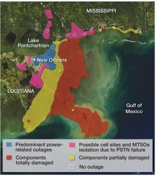
Circles show the locations (cell towers) included in the sample. MTSO stands for mobile-telephone switching office (which connects all individual cell towers to the central office); PSTN for public switched telephone network (which connects landline services).
