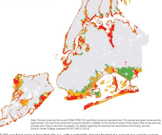
Figure 9.7 100-year flood zones in New York City (i.e., with a probability of being flooded of 1 percent per year) for current and two different ClimAID sea level rise scenarios
