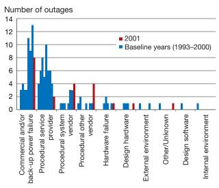
Note: The largest number of telecommunications outages was related to commercial grid and/or service-provider backup power failures.
