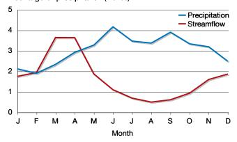
Figure 4.3 Average monthly streamflow discharge and precipitation for the Fall Creek watershed in Central New York
