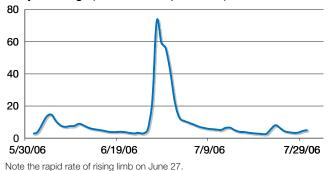
Figure 4.8 Water level of the Susquehanna River at Conklin, New York, during the June 2006 flood
