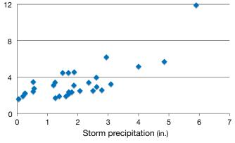
Figure 4.11 Storm rainfall amount and resulting instantaneous peak discharge on Fall Creek, Tompkins County, for the annual peak discharges from 1974 to 2007
