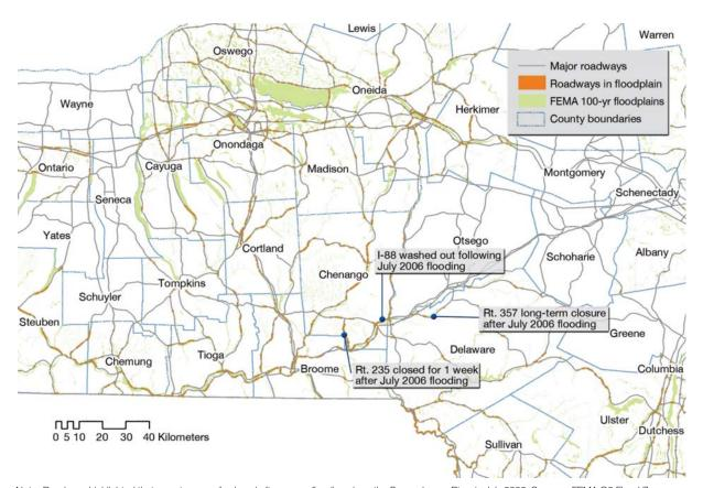
Note: Roads are highlighted that were temporarily closed after severe flooding along the Susquehanna River in July 2006. Sources: FEMA Q3 Flood Zone Data, Census 2000 Railroads, USGS NYS Transportation Coverage
