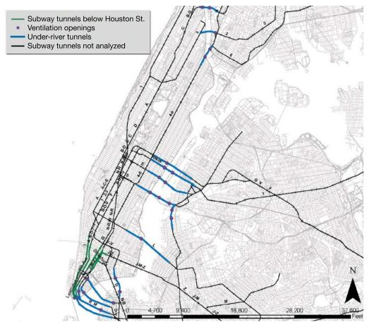
Note: Only the colored segments were considered in the ClimAlD flood analysis. Purple lines are river-crossing tunnels and adjacent segments to the nearest land stations; green lines are analyzed tunnel segments on land, near or beneath flood zones. Subway stations are not shown, but non-station openings subject to potential flooding are indicated by circles. Source: LDEO/Civil Engineering, Columbia University
