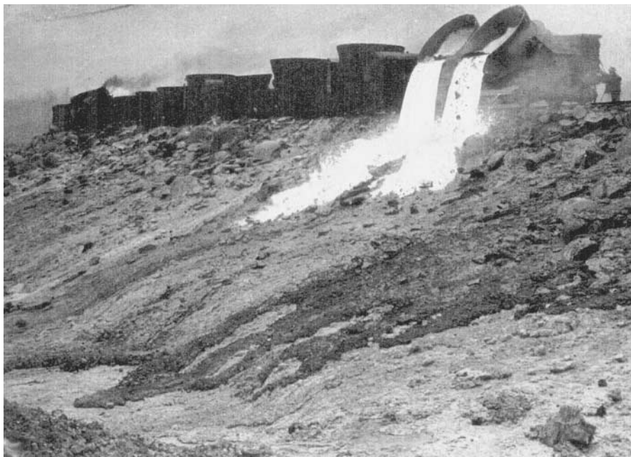
Figure 13: Pouring slag. Although not a Nine Mile Run picture, this was typical of the slag-dumping practices in the valley.
