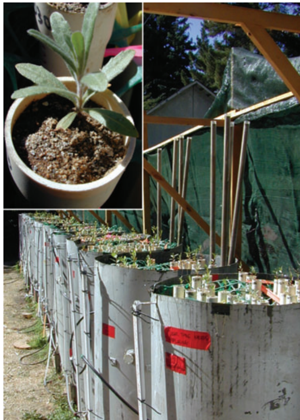
Figure 1. The experimental setup consisted of 20 tanks with seedlings grown in PVC tubes suspended within each tank (inset). Four tanks were randomly assigned to each of five drawdown treatments. Each tank contained individuals of all species tested.
