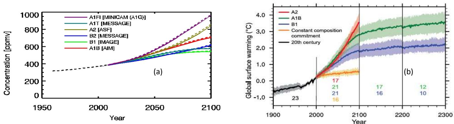
Figure 1. (a) Carbon dioxide concentration of global greenhouse gas emissions scenarios ([http://www.ipcc-data.org/ddc\\_co2.html](http://www.ipcc-data.org/ddc_co2.html)). (b) Average and range (shown by shading) of global temperature change simulated by GCMs given emissions scenarios for the 21<sup>st</sup> century.
