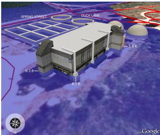
Figure 9: Wastewater Treatment Plant in Hull, MA: Simulated flooding around a critical facility from base flood plus 3.3 feet of sea level rise.
