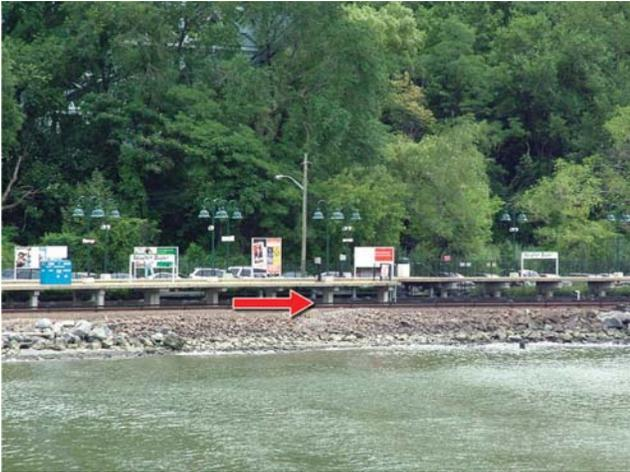
Notes: The red arrow shows the lowest critical elevation, LCE=6.6 feet, of the rail tracks located in waterway zone Z3=9 feet. The elevated concrete structures are the passenger platforms at an elevation near 11 feet. Note the low-lying parking lot in background.
