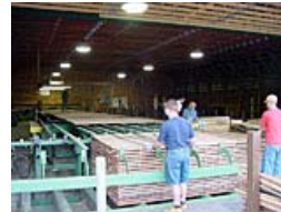
Sticking Green Lumber at the North Mill
