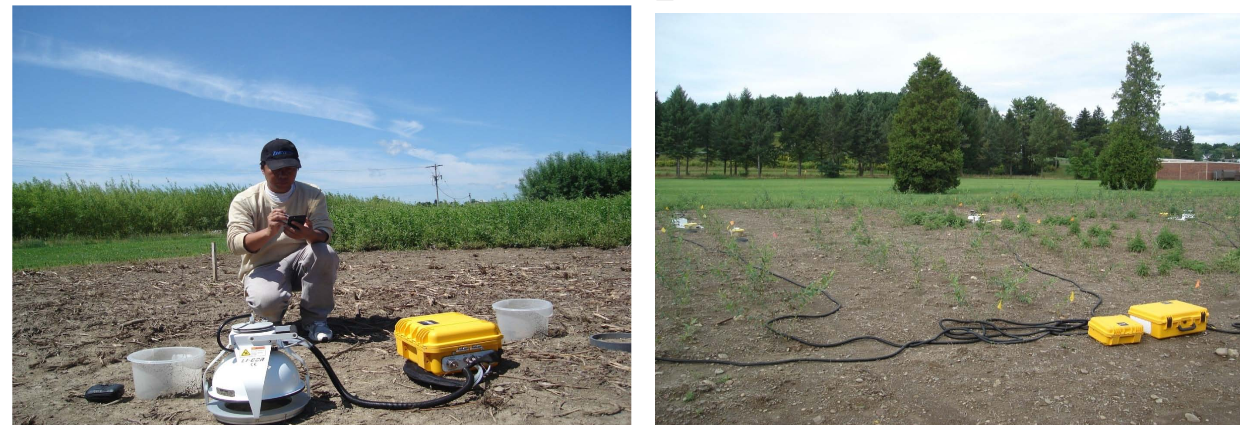
Short term survey measurements using LI-8100 and survey chamber Long term continuous measurements using LI 8100 and multiplexer (LI-8150)
