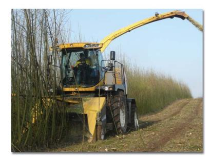
trees up to 15 cm (6 in.) in diameter. No changes are needed to feed rolls or chopper drum on the base unit when using the Coppice Header. Operators can harvest one or two rows at a time, depending on the crop, and can adjust the cutting length from 6 to 66 mm (0.2 to 2.6 in.) to meet end-user specifications.
