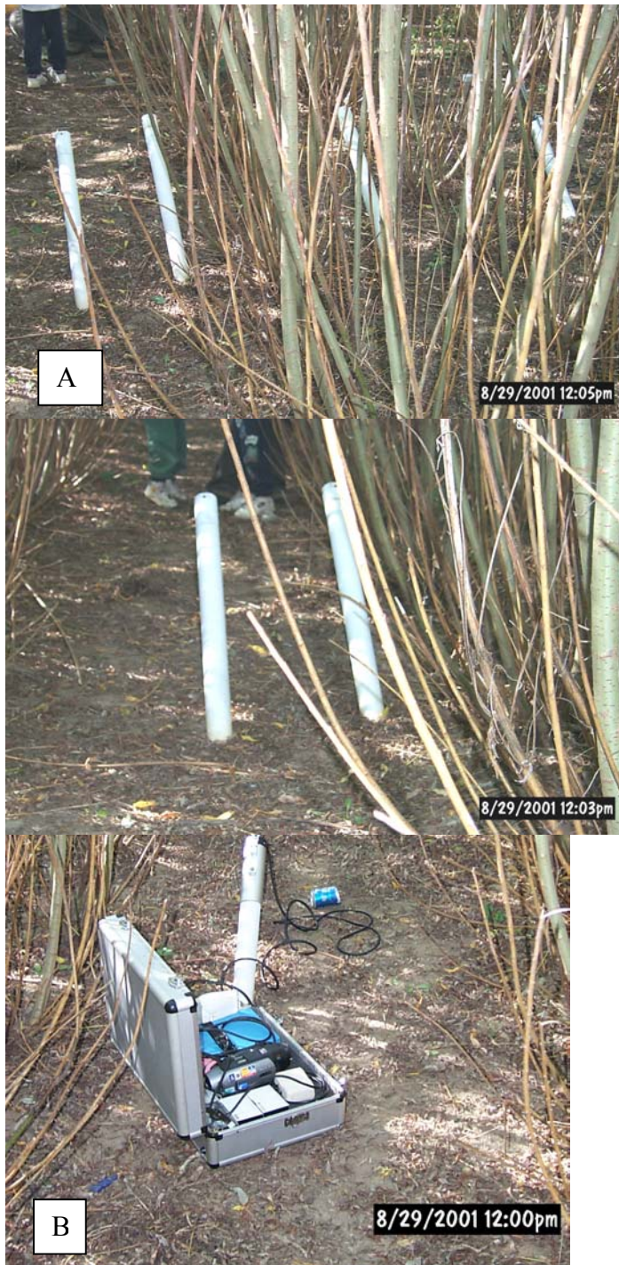
Figure 2. Minirhizotron tubes inserted in willow biomass research plots in Tully, NY. (A) Two tubes located in the 1.5 m space between the willow double rows. (B) Four tubes are inserted across the double row in each of six different plots. (C) The minirhizotron camera inserted and hooked up to recording instruments to collect images belowground.
