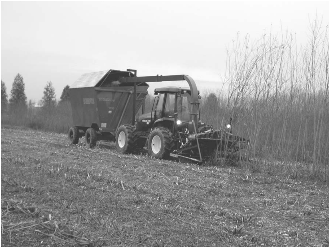
Figure 3. The Bender harvesting willow biomass crops on three-year-old demonstration plots in Tully, NY. (Photo by R. Nissen).
