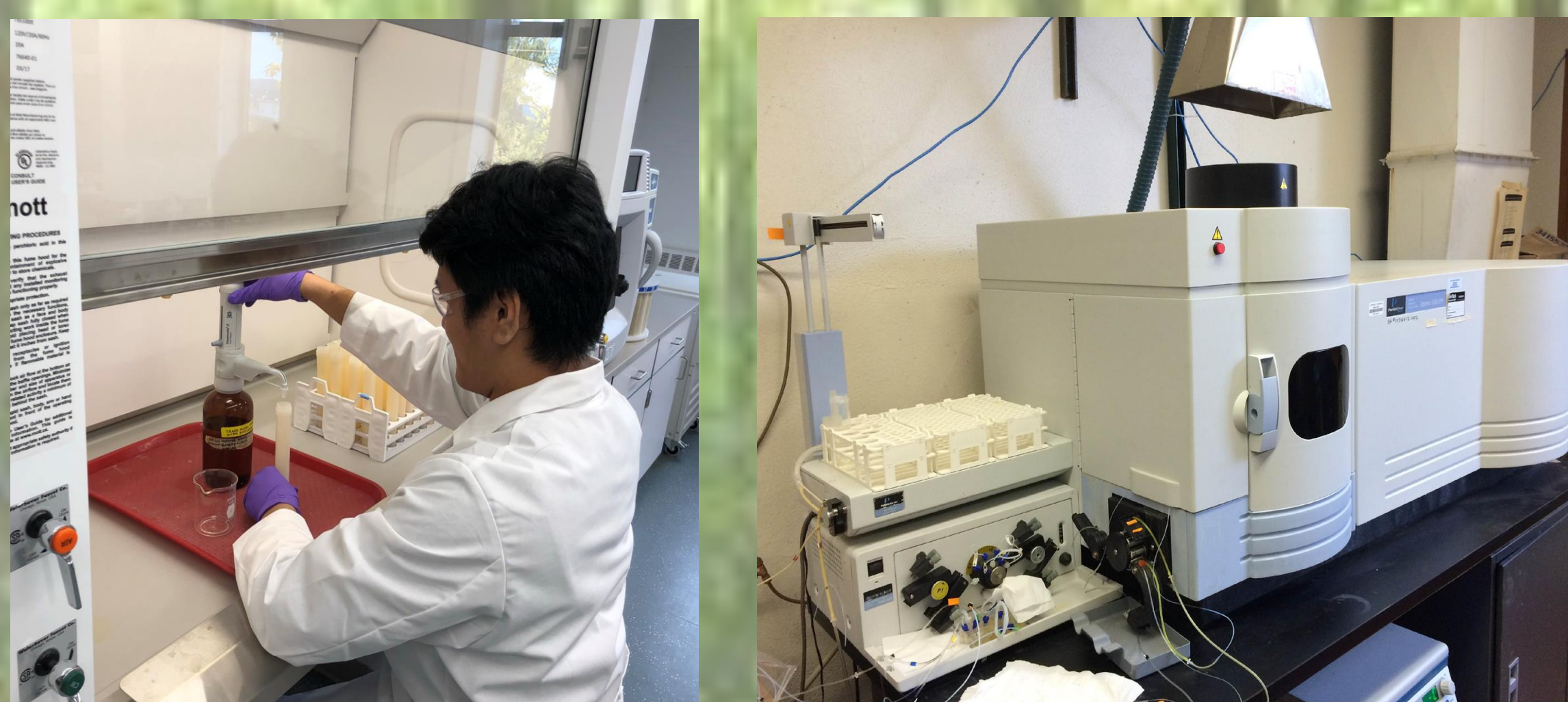
P and other elements were analyzed by Optima 5300 DV ICP-OES (Perkin-Elmer) following an acid-digestion.
