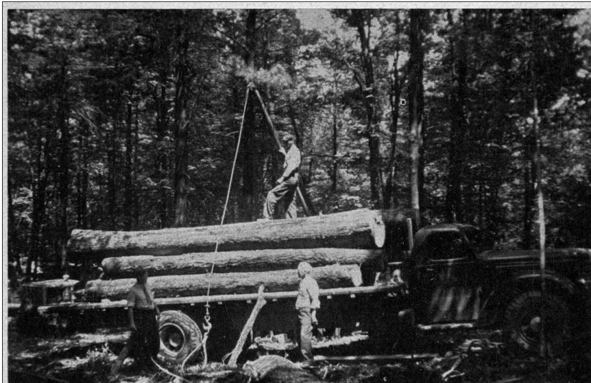
Good-sized white and red oak logs being loaded with A-frame and power take-off from large trucks. These logs are hauled about 55 miles to the sawmill at Ridgefield, Conn.
