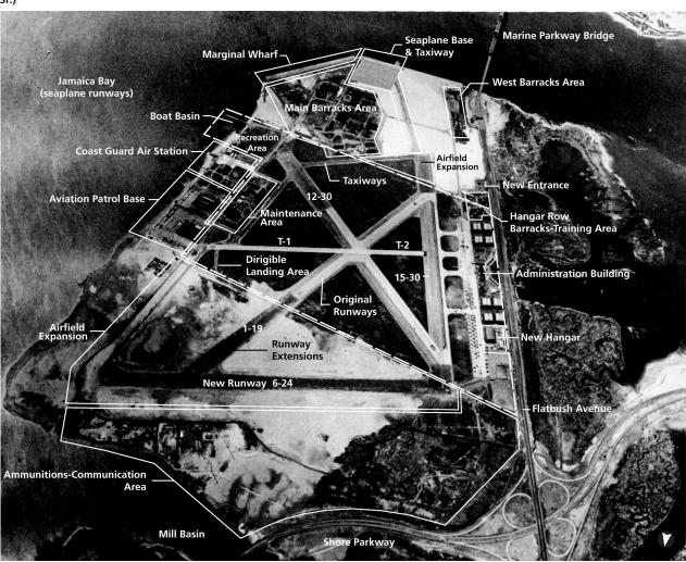
marginal wharf (fig. 1.74). New buildings and other above-ground structures were developed outside of flight paths, which were defined by clear zones approximately 500 feet to either side of each runway and additional areas on the approaches.<sup>36</sup> Given its limited acreage, the Coast Guard made relatively minor additions to its air station at Floyd Bennett Field during the war.
