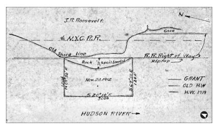
Figure 2.65. Map of J. R. Roosevelt's grant of land under water off the end of River Road illustrating "rockspoil" boat landing constructed by 1919. Notes on the survey stated: "Rock fill made along shore west of N. Y. C. right-of-way from 0 to 30 feet in width used for landing for private boats." ("Department State Engineer and Surveyor Examination of Grant of Land Under Water, August 13, 1919," Hackett Legal Papers, file "Correspondence...1927–1926," Franklin D. Roosevelt Library.)
