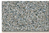
Example of Resin Bound Paving Composite (www.sureset.co.uk)
