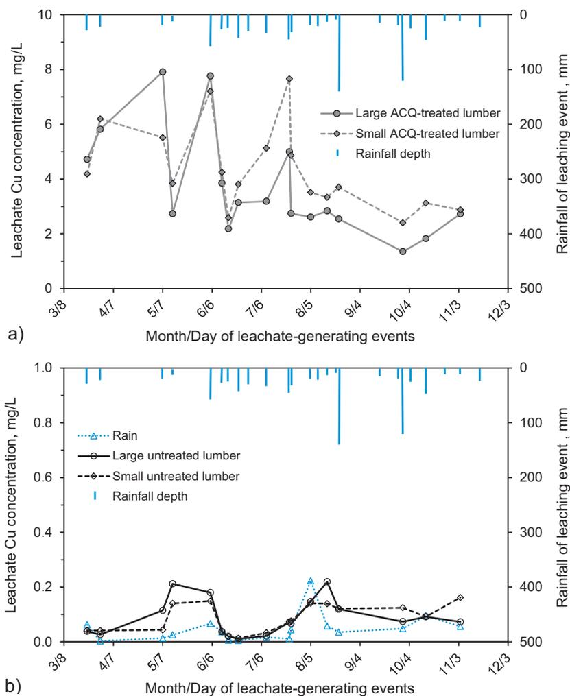
**Fig. 4.** Dynamics of Cu concentration in leachate from ACQ-treated and untreated red pine lumber piles.
