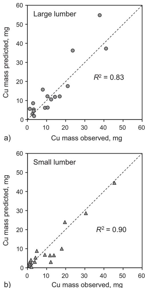
**Fig. 6.** Observed and predicted Cu mass in leachate from the large and small ACQ-treated lumber piles during individual rainfall events.
