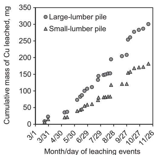
Fig. 7. Cumulative mass of copper leached from two ACQ-treated red pine piles with different lumber sizes over 25 leachate-generating events in 2010.
