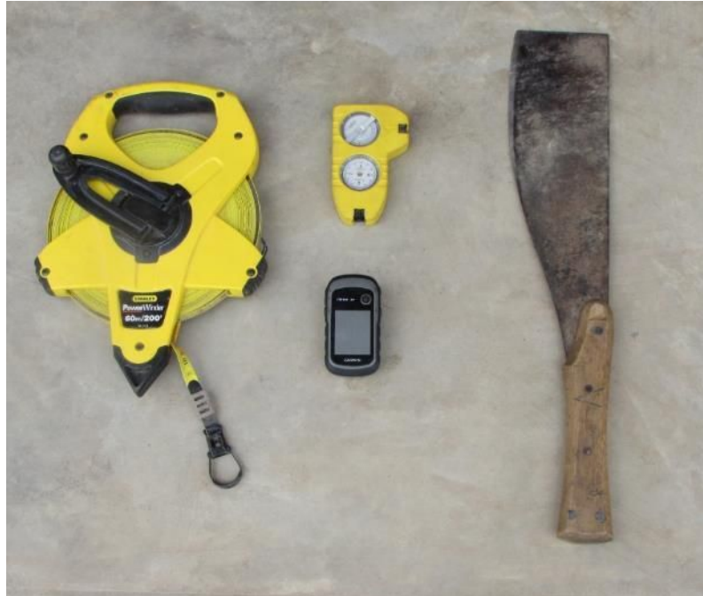
Figure 5: Field equipment used for tamarisk mapping and measurement. 60-meter tape, clinometer, GPS receiver and machete.
