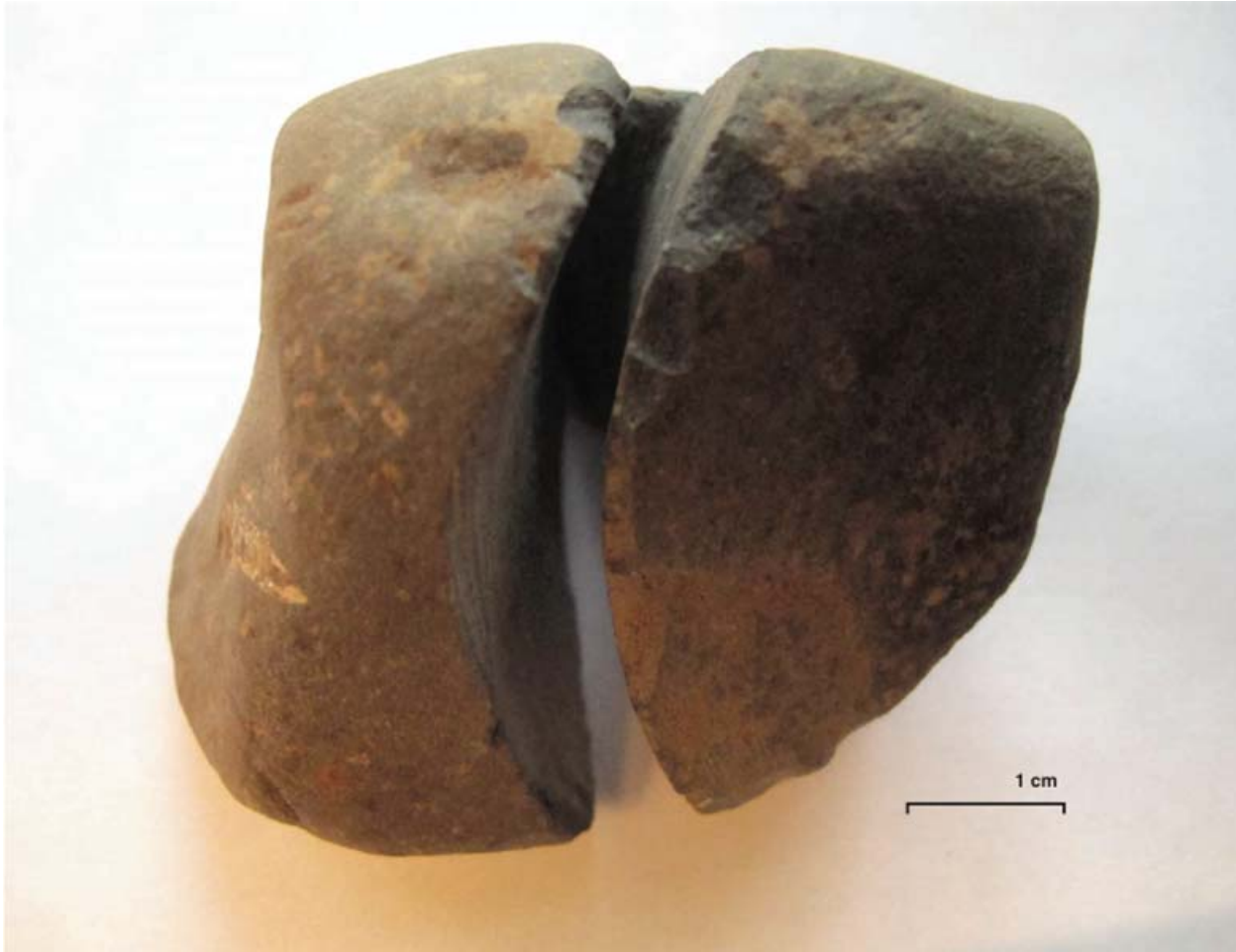
Figure 1. An example of a rock that has been sheared by the rotary corer during coring. The right side of the rock was found in the cored sample and the left side of the rock remained in the wall of the cored hole. The rock broke off before it was shorn completely through; this is visible in the photograph in the upper half of the space between the two sides.
