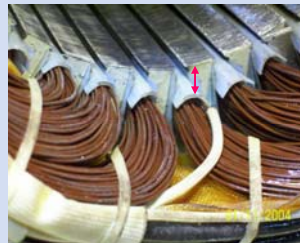
Image of concentric winding that does not use all the slot space available in the stator
