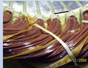
Image of lap winding that shows a complete use of the slot space filled with copper wires to maximize heat dissipation.
