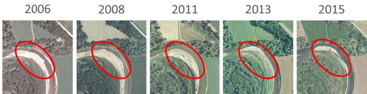
Figure 9. Example Channel Incision and Vegetation Regeneration Along Main Stem of Genesee River
