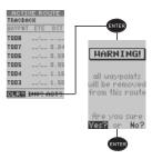
To cancel an active TracBack, highlight the 'CLR' field at the bottom of the active route page and press ENTER. Highlight 'YES' on the warning page and press ENTER again to confirm.
