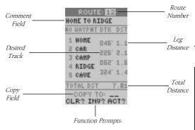
The last form of navigating to a destination with the GPS 12CX is by creating a user-defined route. The GPS 12CX lets you create and store up to 20 routes of 30 waypoints each.
