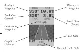
The GPS 12CX's Highway Page provides graphic steering guidance to a destination waypoint, with a greater emphasis on the straight-line desired course and the distance and direction you are off course. The bearing and distance to a waypoint—along with your current track and speed—are displayed at the top of the screen.
