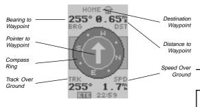
Whenever you select a destination waypoint, the GPS 12CX provides graphic steering guidance with the Compass Page (the default navigation page). The "compass ring" in the middle of the page acts much the same as the "compass tape" at the top of the Position Page, it provides a graphic representation of your present track (TRK). The "pointer" is a graphic representation of the direction or bearing (BRG) to the destination waypoint, and points in the direction you need to travel.
