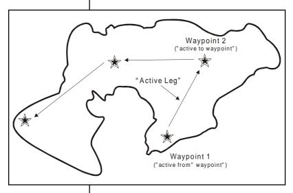
Routes are broken down and navigated in smaller segments called "legs". The waypoint you are going to in a leg is called the "active to" waypoint and the waypoint immediately behind you is called the "active from" waypoint. The line between the "active to" and the "active from" waypoint is called the "active leg".
