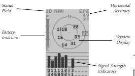
The GPS 12CX's Satellite Page displays the status of various receiver functions. The status information will help you understand what the GPS 12CX is doing at any given time, and will tell you whether or not the receiver has calculated a position fix.
