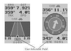
The 'ETE' field, located at bottom center on both pages, is a user-selectable field that allows you to display a variety of navigation values for your trip.
