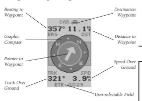
The Compass Page provides better steering guidance than the Highway Page for travel at slower speeds (e.g., walking), travel with many directional changes and when it's not necessary to follow an exact course.
