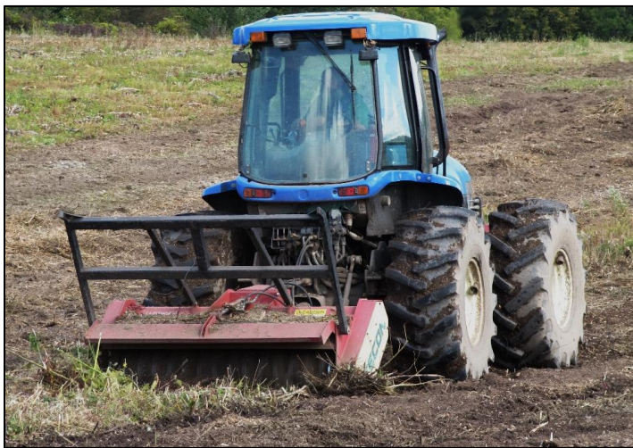
Figure 3: A PTO-driven forestry mulcher grinding cut willow stools and roots so they can decompose back into the soil. The areas around the tractor show previous willow plantings that have already been ground using this method.
