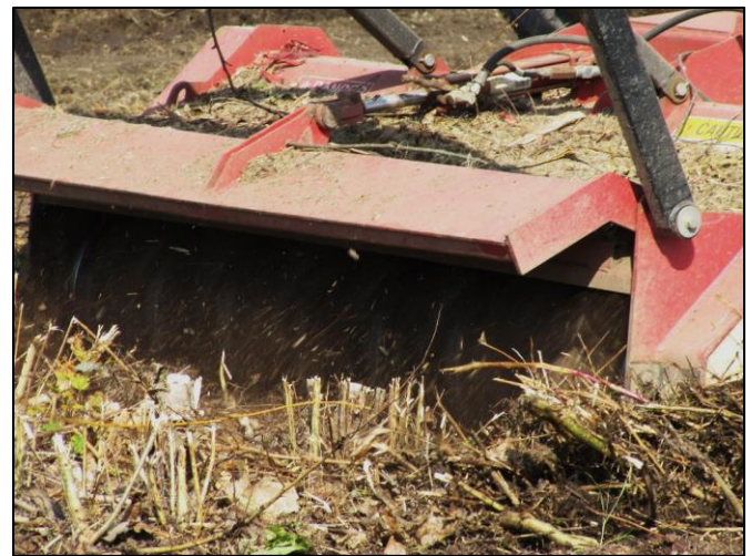
Figure 4: Close-up image of a forestry mulcher grinding cut willow stools after harvest. The drum spins at high speeds and the heavy-duty tines chop and grind the woody material and fibrous roots left in the field after harvest.
