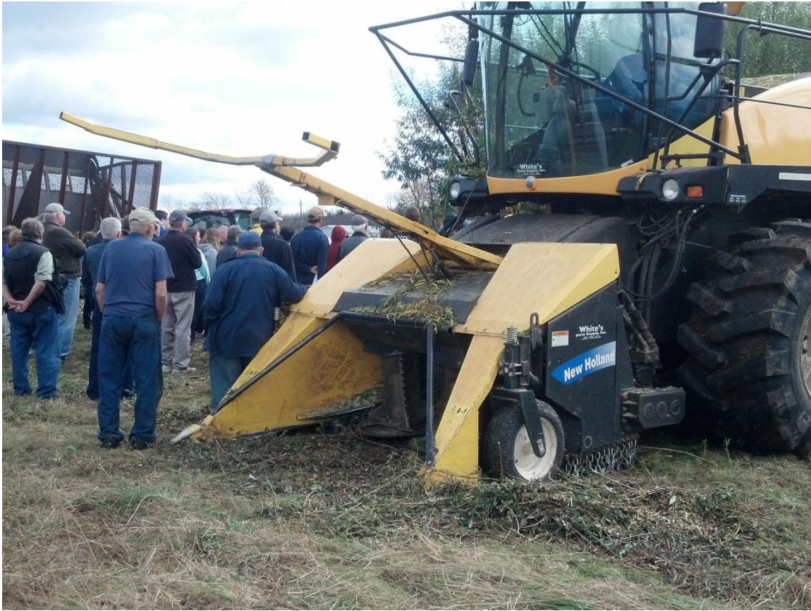
Image 11: Specially designed New Holland shrub willow cutter head on forage harvester
