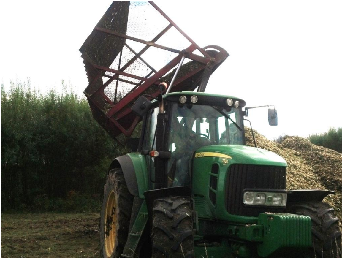
Image 13: Emptying dump wagon onto chip pile at harvest site for short-term storage before transport to ReEnergy Lyonsdale biopower facility
