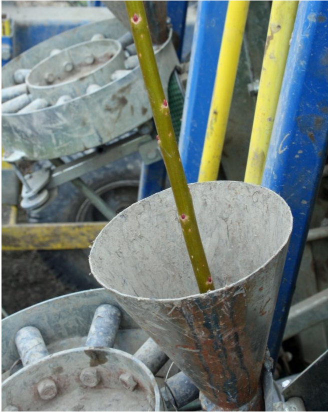
Image 5: Feed mechanism on step planter where shrub willow “whips” are fed into the plant and subsequently cut into down 6 – 8 inch cuttings during planting
