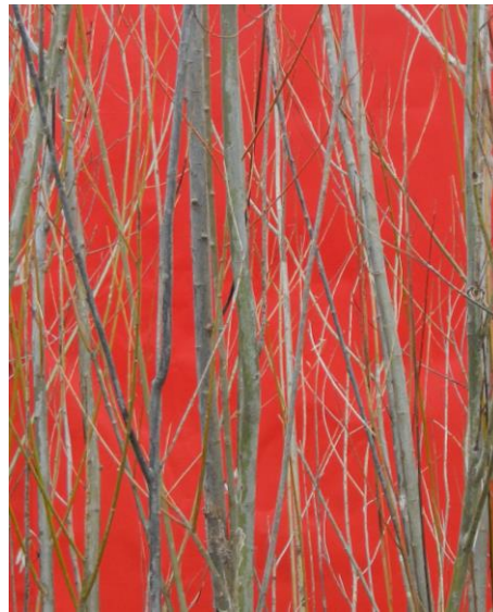
Figure 4 – Photo of a shrub-willow living snow fence in winter. Plant stems are pictured in the foreground, in front of a red backdrop highlighting the optical porosity (open space) of the fence Image by SUNY ESF
