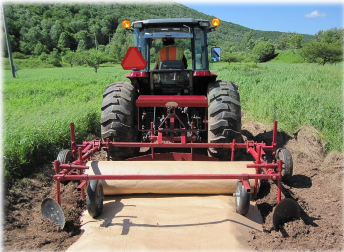
A paper landscape fabric is applied to a prepared planting strip using a roller attachment
