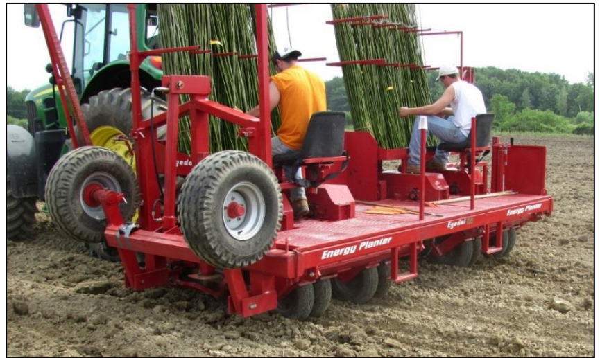
Figure 3: Specialized willow planters plant two rows of willow cuttings from long whips. Two models of planters are available for rental or custom rates.
