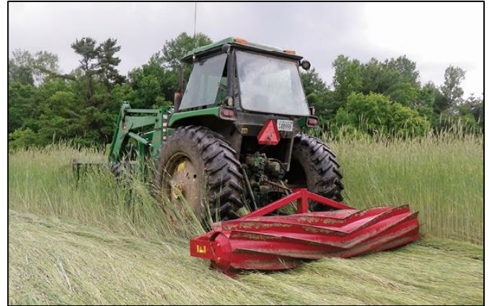
Figure 1: Terminating a cover crop in spring using a roller-crimper. (Image courtesy of Rodale Institute)
