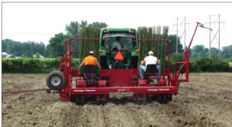
Figure 1. Planting a willow crop in northern New York State using a specialized double-row willow planter. Photo: SUNY-ESF .
