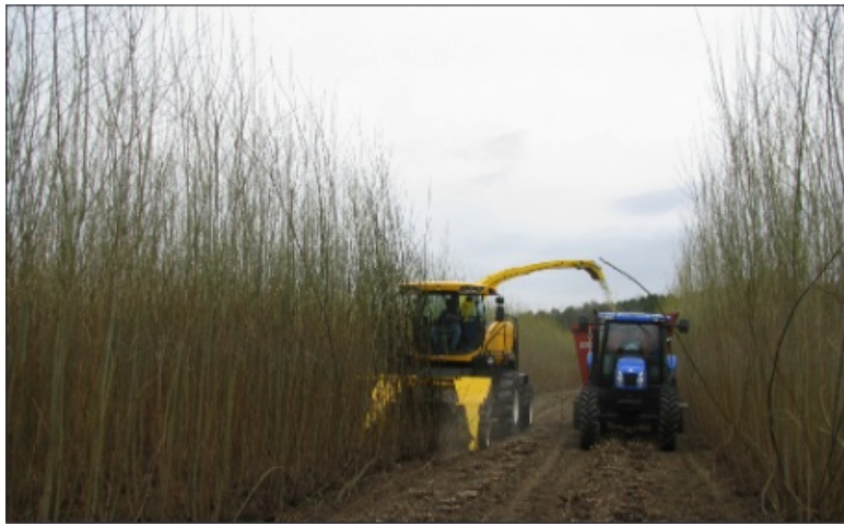
Figure 2. Willow in the Northeast is commonly harvested using a newly developed system developed by SUNY-ESF, New Holland Agriculture, and partners. Photo: SUNY-ESF .
