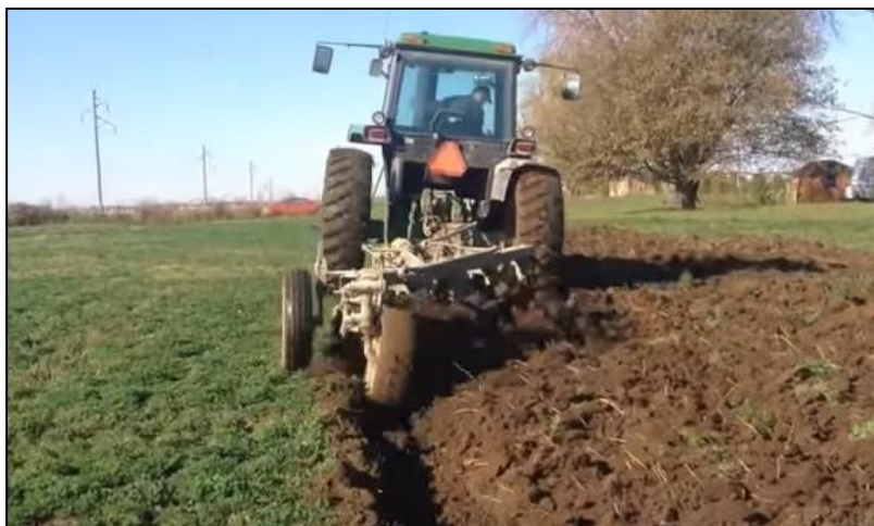
Figure 4: A moldboard plow turns the soil and breaks up sod and compaction before discing. (Image courtesy of Iowa Dairy Boys)
