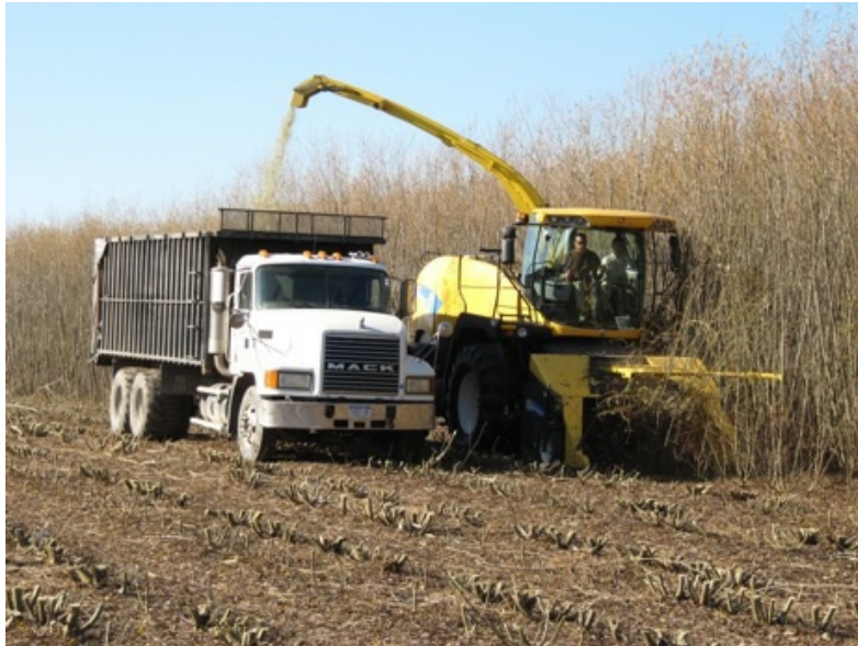
Harvesting willow biomass crops in Auburn, NY with a New Holland single-pass cut-and-chip harvester. Photo: Timothy Volk.
