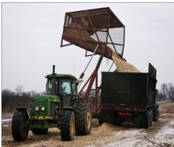
Figure 3. After harvest, willow chip are transferred into a truck from transport to short-term storage or an end user. Photo: SUNY-ESF .
