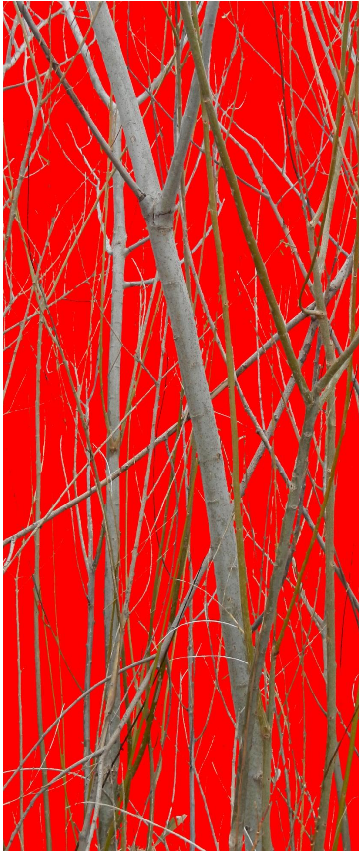
Figure 33: Optical porosity photo sample from living snow fence Tully-C-willow-6 showing stem morphology of shrub-willow variety Sherburne
