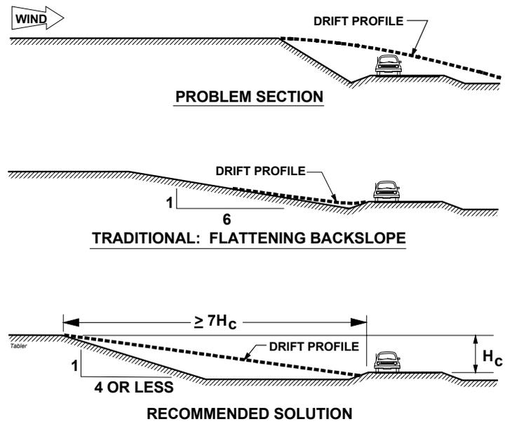
**Figure 8.23. Guidelines recommended in Figure 8.22 maximize snow storage in cut and reduce possibility that drift will encroach on roadway.**
