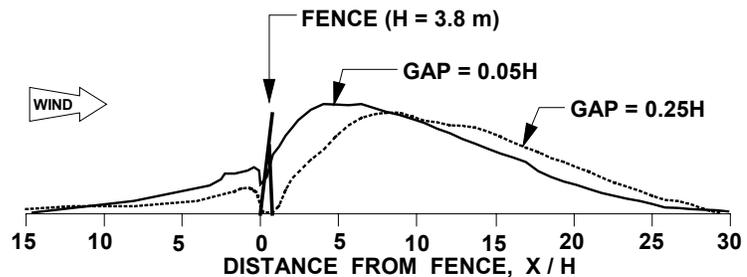
**Figure 3.48. Effect of bottom gap on snow storage, as determined from field studies (Tabler 1994).**
