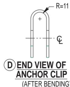
Ⓓ END VIEW OF ANCHOR CLIP (AFTER BENDING)
