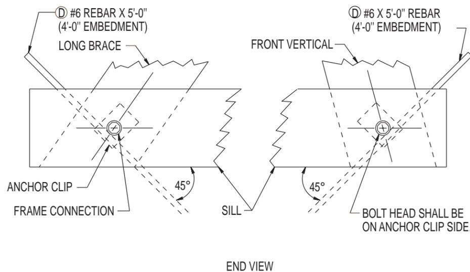
(D) ANCHOR CLIP CONNECTION DETAIL
