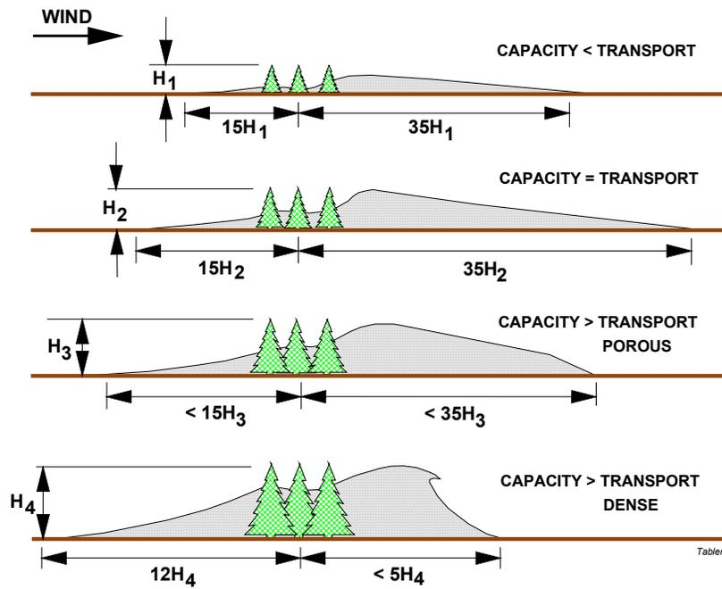
**Figure 5.32. Minimum setback for moderate to severe snow transport, and placement of structural fence if required.**
