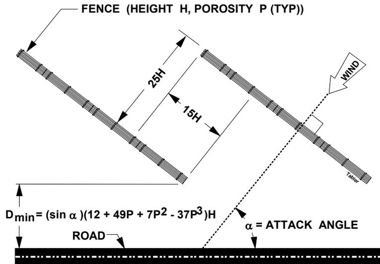
**Figure 6.70. Swept-back herringbone fences to be used where winds are aligned with the road centerline (Tabler 1994).**
