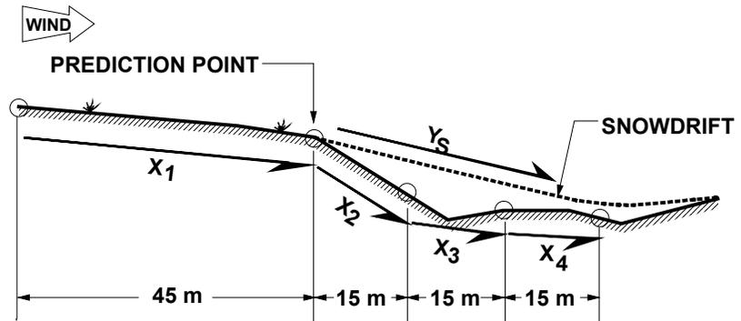
**Figure 8.2. One of the larger topographic accumulation areas used to derive Equation (8.1)(Tabler 1994).**
