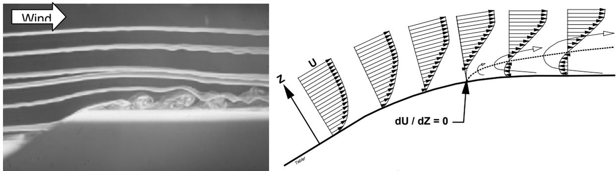
**Figure 8.13. "Separation" of airflow at the top of an embankment causes the eddy area where blowing snow is deposited.  $dU/dz$  is the vertical velocity gradient. Upper left view uses smoke for flow visualization in a wind tunnel (courtesy University of Wyoming). Lower right view shows 1:30 scale model of dam.**
