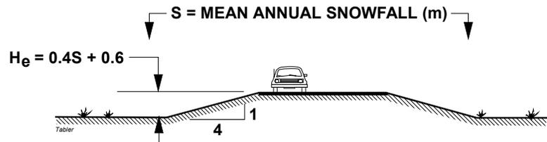
**Figure 5.12. Recommended treatment for high fill sections.**
