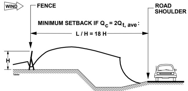
**Figure 5.21. The best location for a snow fence may be farther from the protected area than the minimum setback.**
