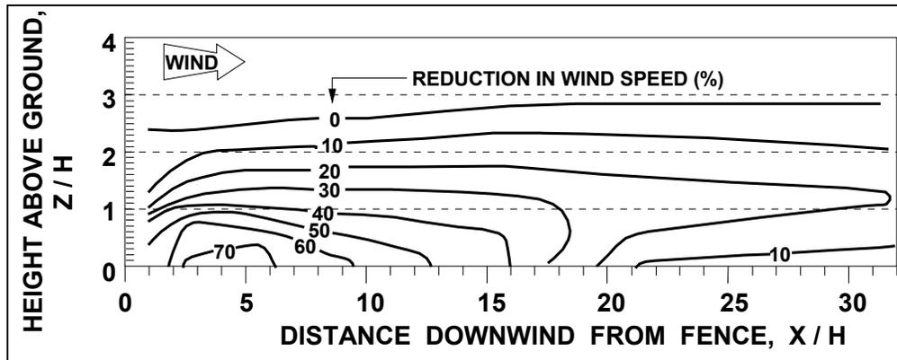
**Figure 3.30. Wind speed reduction contours on the lee side of a 50% porous snow fence with height  $H$  (Tabler 1986). Contour values are percent of ambient (undisturbed) wind speed at an equivalent height.**
