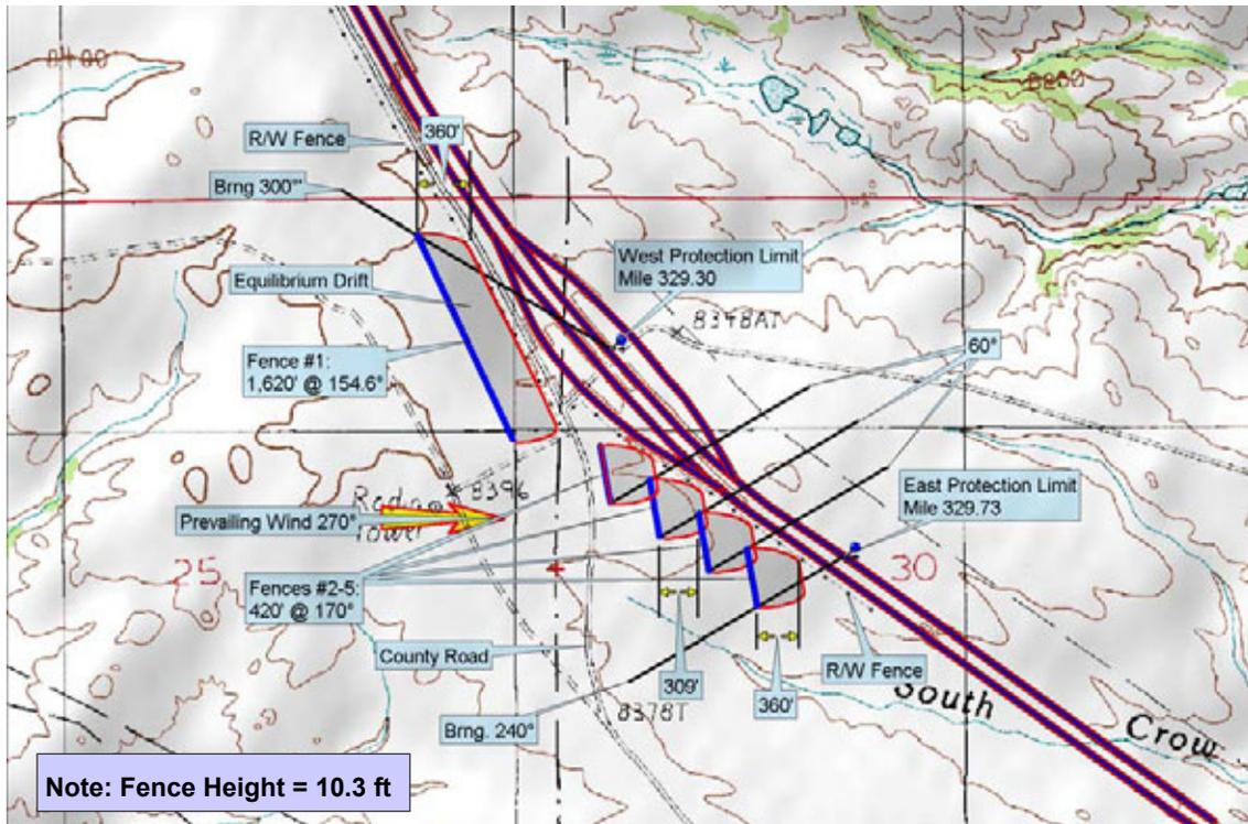
Figure 6.89. Example illustrates preliminary layout of a snow fence system using DeLorme software. © 2002 DeLorme ([www.delorme.com](http://www.delorme.com)) XMap® 3.5 and 3-D TopoQuads® 1.0. [ 1 m = 3.28 ft]
