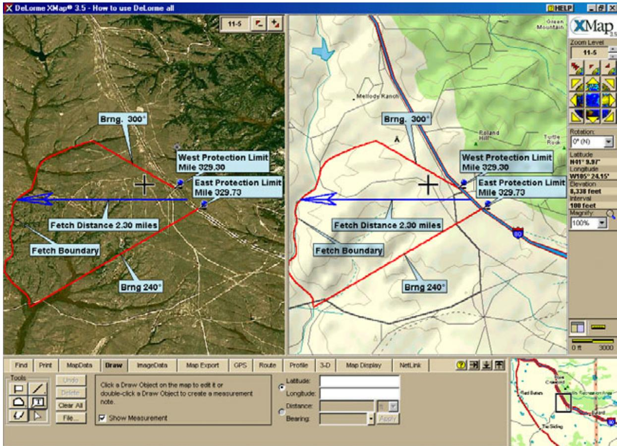
**Figure 6.91. Computer “print screen” image showing how 10-meter satellite imagery can be used in conjunction with XMap<sup>®</sup> and 3-D TopoQuads<sup>®</sup> to determine fetch distance for the example in Figure 6.89. © 2002 DeLorme ([www.delorme.com](http://www.delorme.com)) XMap<sup>®</sup>3.5, 3-D TopoQuads<sup>®</sup>1.0, and Sat 10 Satellite Imagery.**
