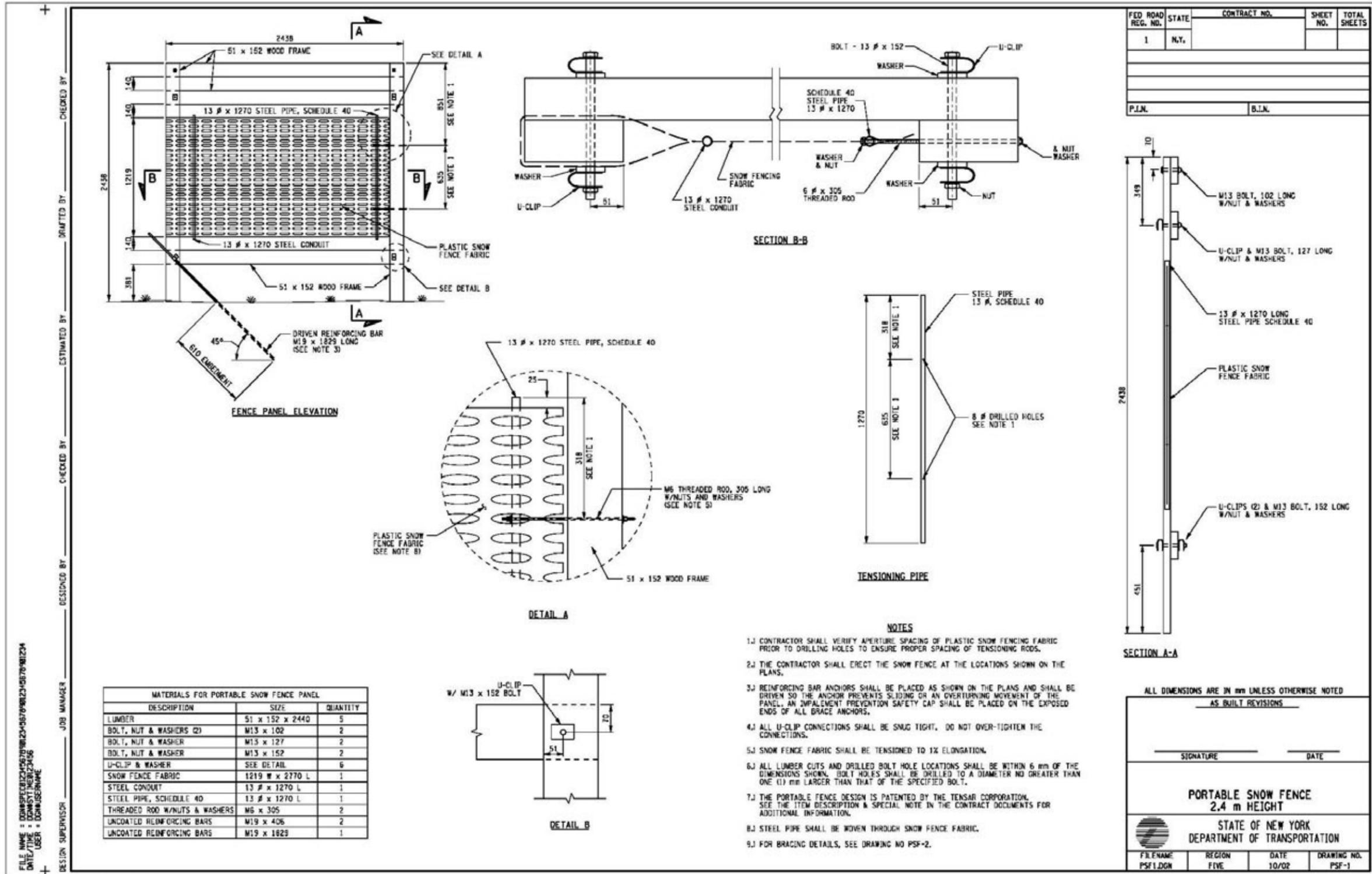
Figure 6.55. Standard Plan for the 2.4-m (8-ft) portable fence, Sheet 1 of 2. Figure courtesy of the New York State Department of Transportation.
