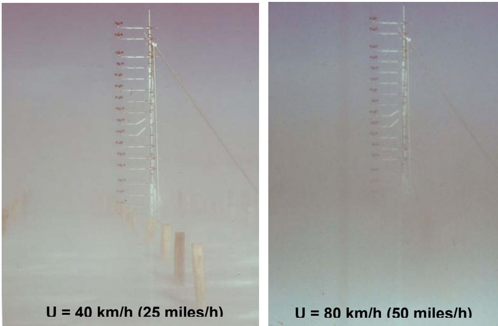
**Figure 3.10. Visual demonstration of how the vertical distribution of blowing snow changes with wind speed  $U$ . This array of anemometers, spaced 30 cm (12 in.) apart, was set in a field of wood posts 1.2 m (4 ft) tall (Tabler 1986).**
