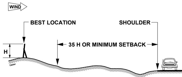
**Figure 6.75. Fences on embankment slopes should be spaced as shown in this illustration (Tabler 1994).**
