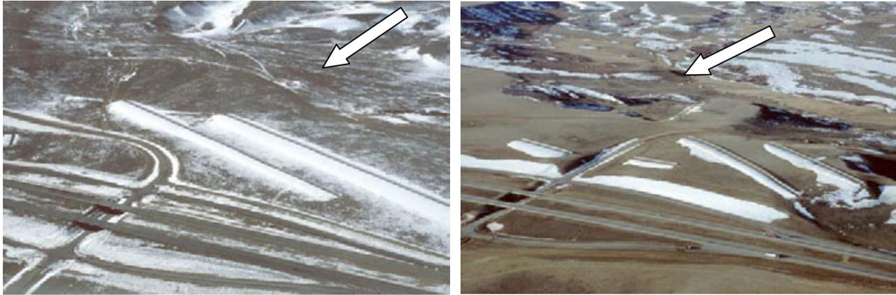
**Figure 8.10. Examples of good (upper left) and poor (upper right) layout for grade separations. Arrows indicate wind directions. Recommended conceptual design (right, from Tabler 1994) allows snow fences to be installed to protect structure.**
