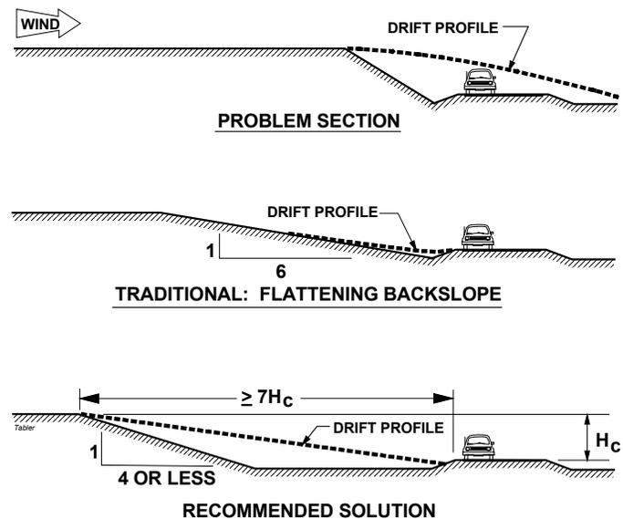
**Figure 5.6. Proposed section for cuts to prevent drift encroachment where upwind terrain is flat or slopes downward toward the road (Modified from Tabler 1994). Dimensions are in meters.**
