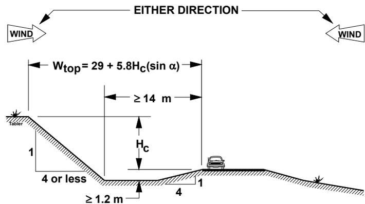
**Figure 8.25. Snow storage versus cut height for 4H:1V backslopes, using cross-section in Figure 8.24.**
