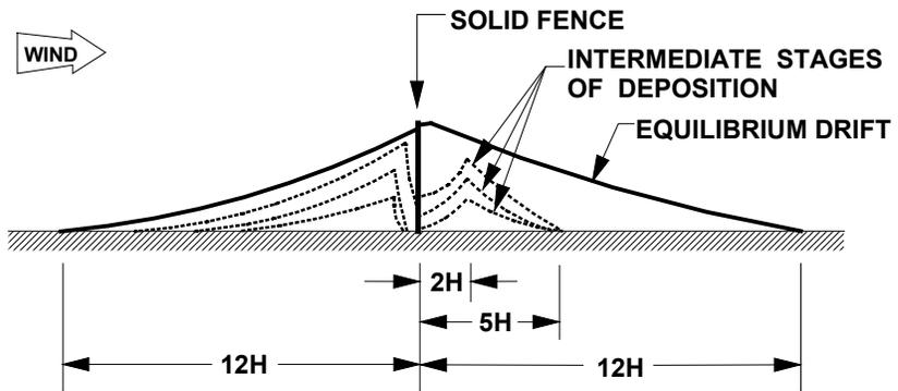
**Figure 3.38. The vortex on the upwind side of this solid barrier prevents deposition immediately upwind of the fence until the snow depth reaches about  $0.6H$  (Tabler 1994).**
