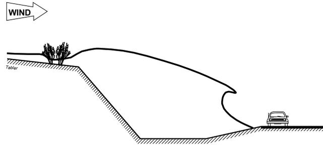
**Figure 7.9. Shrubs planted at the top of a cut can be used in place of taller barriers placed farther upwind. Snow transport must be accurately determined, however, if the risk of drift encroachment is to be acceptable. (Drawing from Tabler 1994).**
