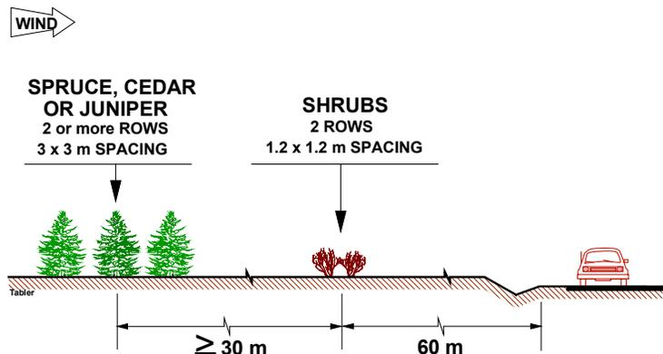
Openings in living fences can cause deep drifts to form downwind and should be avoided (Figure 5.34). Gaps caused by tree mortality should be sealed off with non-porous structural fence until replacement vegetation is established.
