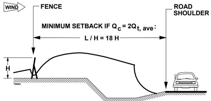
**Figure 6.73. Taking into account the additional snow storage in this cut section reduced the required setback distance to 18H.**
