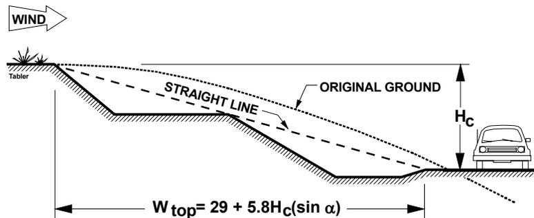
**Figure 8.28. Example of cuts designed according to the recommendations in section 8.8.2.3.**
