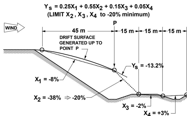
**Figure 8.4. Illustration of how Equation (8.1) is used to generate a snowdrift profile (Tabler 1994).**
