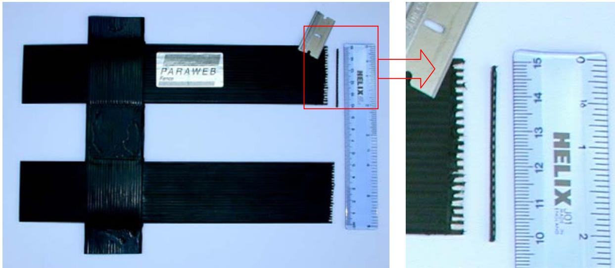
**Figure 6.48.** PARAWEB<sup>®</sup> fencing consists of polyester fibers encased in a polymer sheath. A cross section is shown between the top web and the ruler, and the right ends of the webbing have been shaved to show white fibers.
