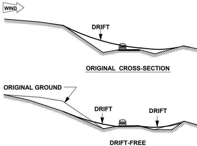
**Figure 8.21. This successful cross-section modification, designed using the snowdrift prediction model, illustrates how geometry on the downwind side of centerline must sometimes be modified to eliminate the drifting problem (Tabler 1975).**
