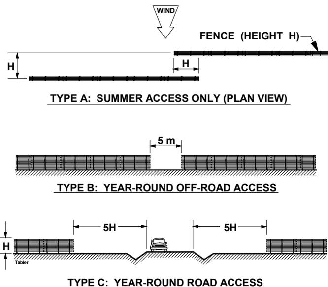
**Figure 6.84. Opening in fence similar to Type A in Figure 6.83. Fence height is 3.8 m (12.4 ft)**
