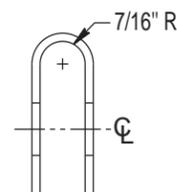
(D) END VIEW OF ANCHOR CLIP (AFTER BENDING)
