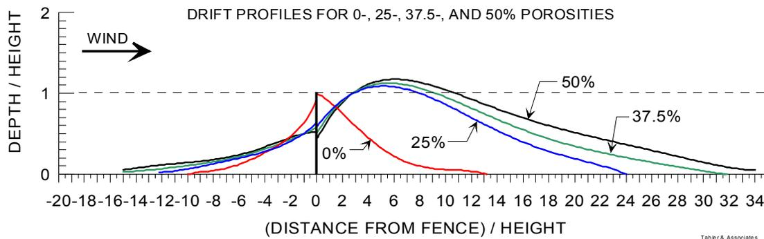
**Figure 6.2. Equilibrium drift profiles for selected fence porosities.**
