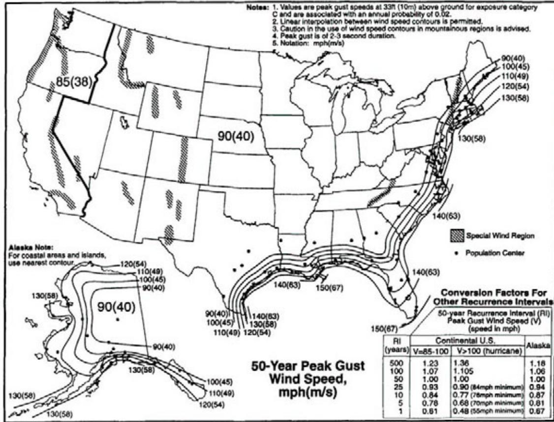
Figure 6.60. 50-year peak gust wind speed map (Peterka, J. A. and S. Shahid 1998. Design gust wind speeds in the United States. *Journal of Structural Engineering* 124 (2): 207-214). ©Copyright 1998 ASCE ([www.pubs.asce.org](http://www.pubs.asce.org)). Reproduced with permission of publisher.
