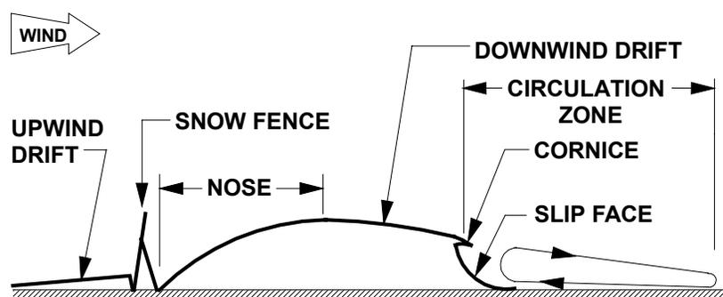
**Figure 3.32. Slip face and cornice behind a 3.8-m (12.4-ft) snow fence (Tabler 1994). Drift is approximately 3.7 m deep at the cornice.**
