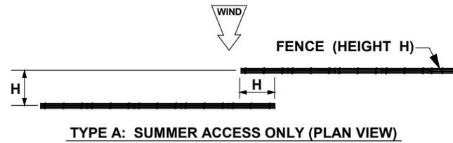
**Figure 5.25. Guidelines for openings in fence lines (Tabler 1994).**
