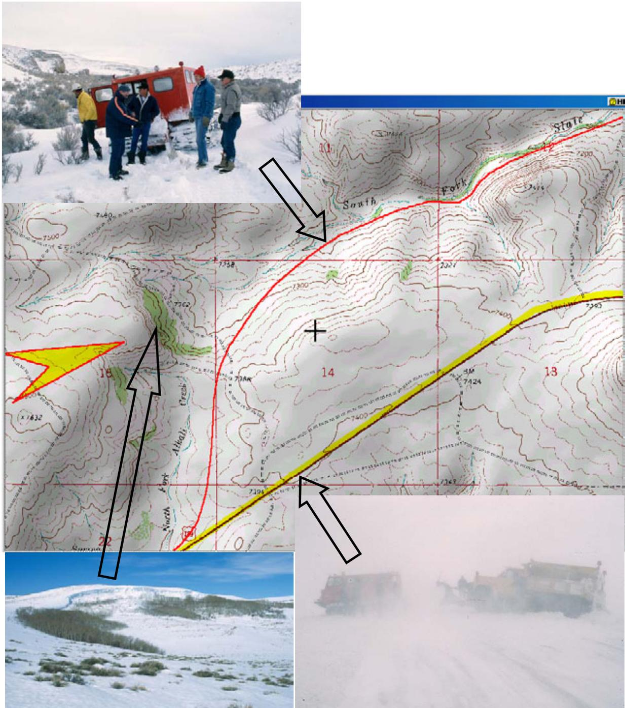
**Figure 8.6.** Comparison of blowing snow conditions on alternate routes shows importance of selecting sheltered locations. Yellow arrow indicates wind direction. Map © 2002 DeLorme ([www.delorme.com](http://www.delorme.com)) XMap® 3.5 and 3-D TopoQuads® 1.0.
