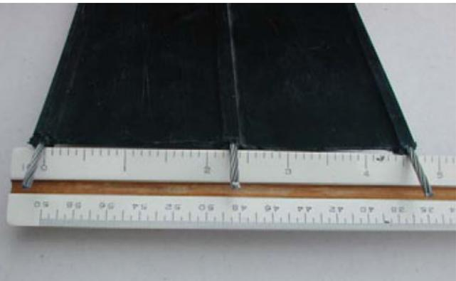
**Figure 5.29. Composite polyethylene / stranded steel wire fencing material (Centaur HTP<sup>®</sup>). Lower right photo courtesy of Perma-Rail<sup>®</sup> International. (Upper left from Tabler 1994).**
