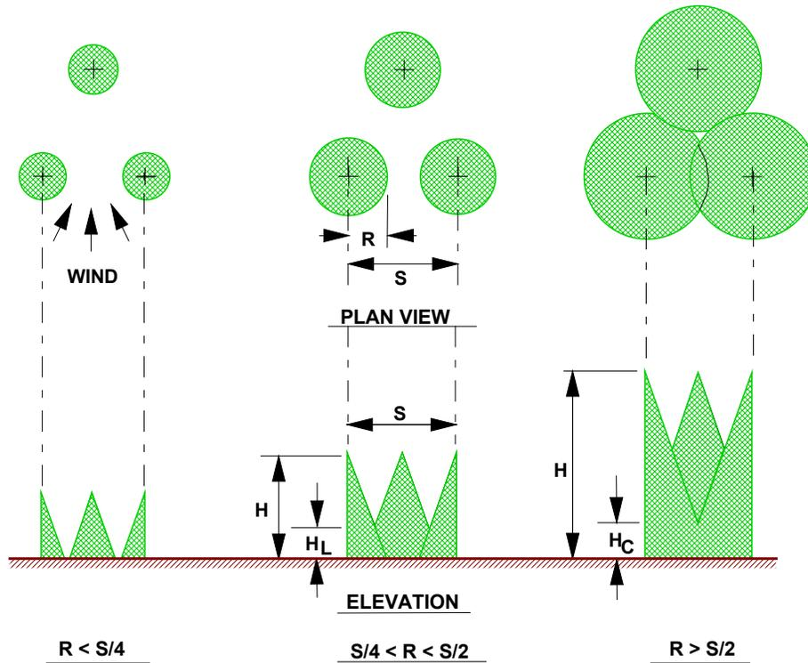
**Figure 7.3. Model of living snow fence (spruce trees) used for computer simulation of porosity, snow-trapping efficiency, and drift length in relation to tree height, spacing, and snow transport (Tabler 1994).**
