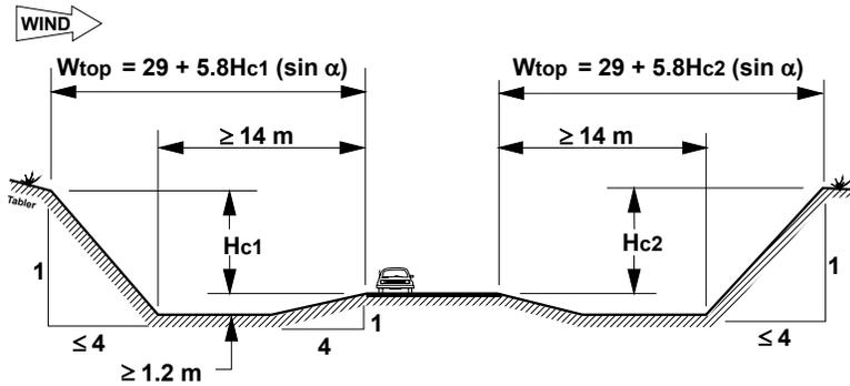
**Figure 5.7. Proposed guidelines for through-cuts (Modified from Tabler 1994).**
