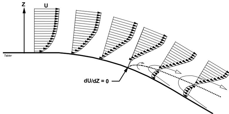
**Figure 3.25. Stages of drift growth in a topographic deposition area (Tabler 1975b).**
