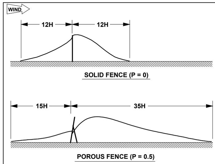
**Figure 3.50. Length of the downwind drift as a function of fence porosity (Tabler 1994).**
