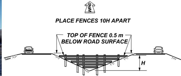
**Figure 6.79. Median fences should be spaced 10 times their greatest height (right from Tabler 1994).**
