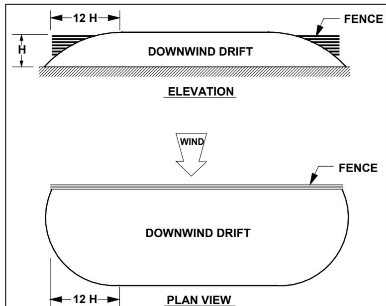
**Figure 3.44. Length of an equilibrium downwind drift as a function of distance from the end of a 50%-porous fence on flat ground (Tabler 1980a).**
