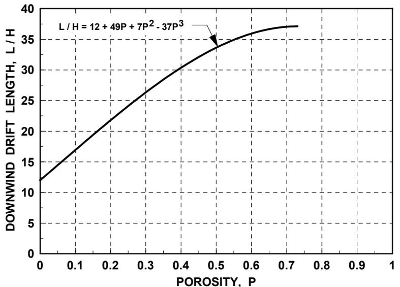
**Figure 3.51. Snow storage capacity of the downwind drift as a function of fence porosity (Tabler 1994).**
