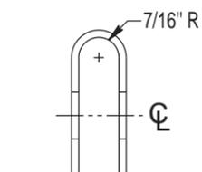
(D) END VIEW OF ANCHOR CLIP (AFTER BENDING)
